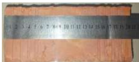
Fig.3. Measuring the dimensions of bricks. The bricks volume was then determined using the following equations.
